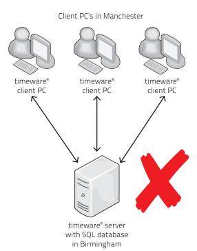
In this example we have client PC's that are located in Manchester and a timeware® server in Birmingham. This setup would cause a massive amount of problems with connectivity that would result in an unusable system. It is NOT recommended to have the client PC's connecting over long distances. Instead, it is recommended to have the client and server be on the same local network.
